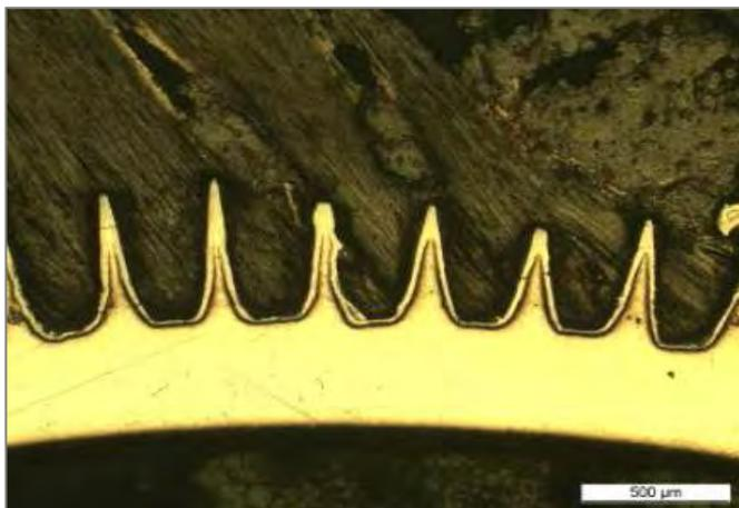
Fig. 7: Cross section of active metal cast CFC/Cu interface.
