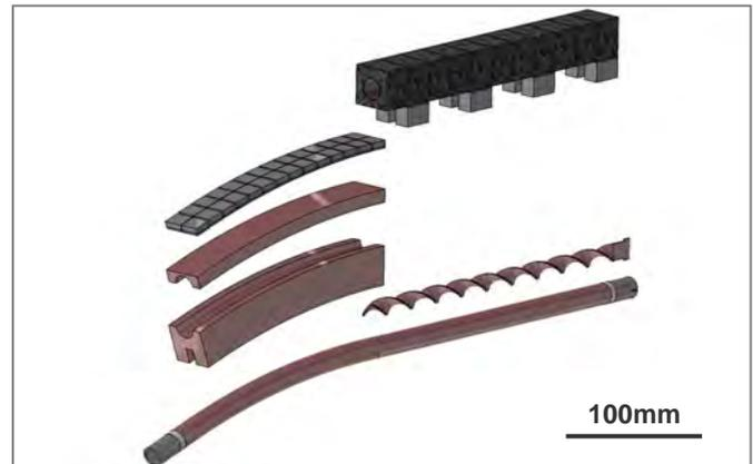
Fig. 3: Design of a single VT mono flat tile heat flux unit.
