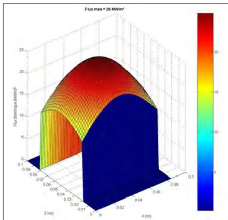
Fig. 21: Estimated heat flux pattern deposition (MW/m<sup>2</sup>).
