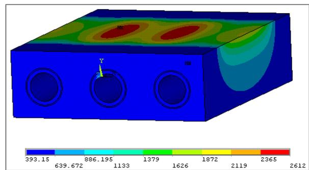
Fig. 22: Calculated surface temperature for 20 MW/m<sup>2</sup> average absorbed heat flux and 25 MW/m<sup>2</sup> maximum incident heat flux.
