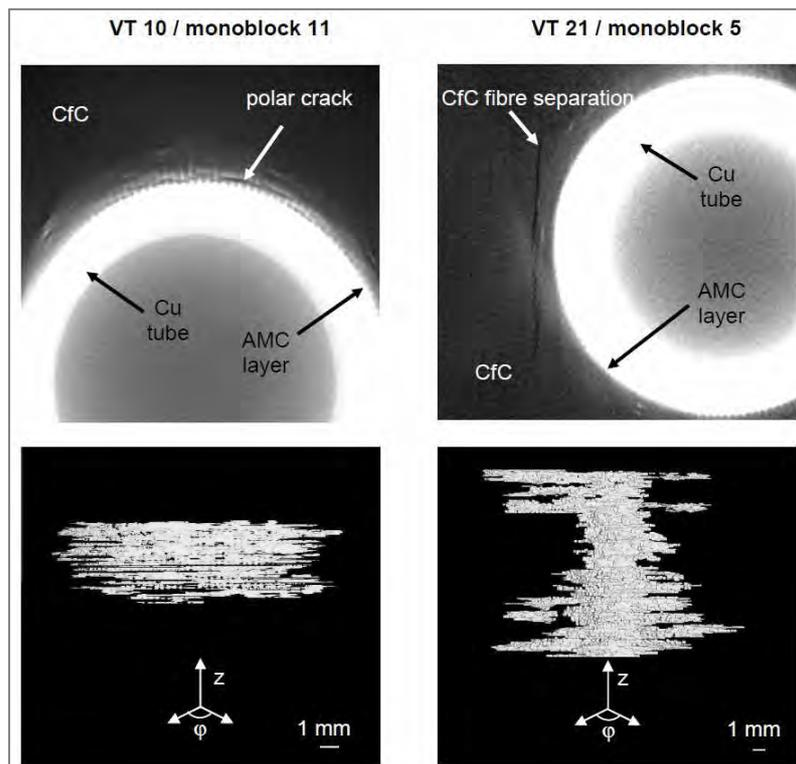
Fig. 13: Results of CT of two defect indications observed by PTT. The cross section slice (top) and the shape of the defect (bottom) are shown for VT10/monoblock 11 (left) and for VT21/monoblock 5 (right).
