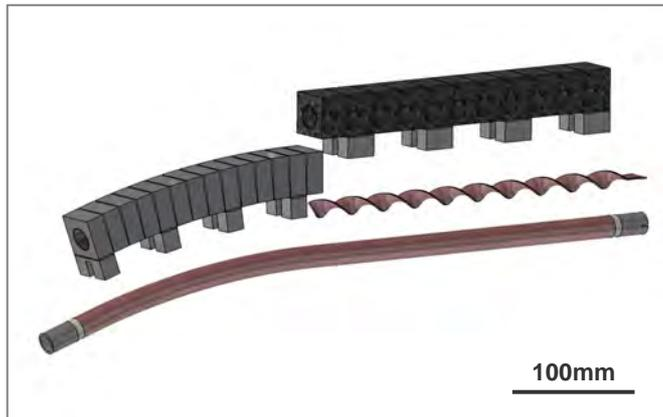
Fig. 2: Design of a single VT full monoblock heat flux unit.
