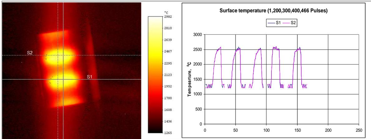
Fig. 20: Measured surface temperature at 20 MW/m<sup>2</sup> average absorbed heat flux and 25 MW/m<sup>2</sup> max. incident heat flux.
