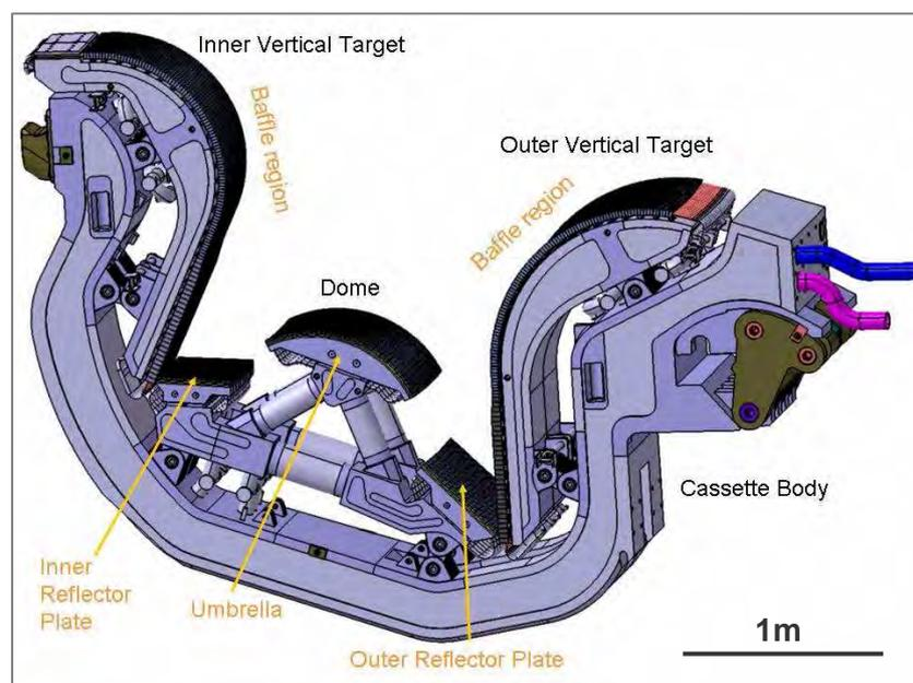
Fig. 1: Schematic view of the ITER divertor.
