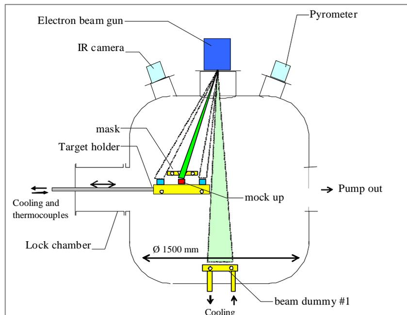
Fig. 17: Schematic view of TSEFEY-M vacuum chamber.
