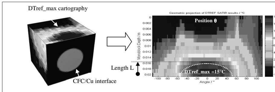
Fig. 15: Geometric projection of the three DTref\_max cartographies of the monoblocks #11 (VT4 prototype) at the CFC/Cu interface to define the defect position  $\theta$  ( $=0^\circ$ ) and axial length L ( $1/5L_{\text{monoblock}}$ ).
