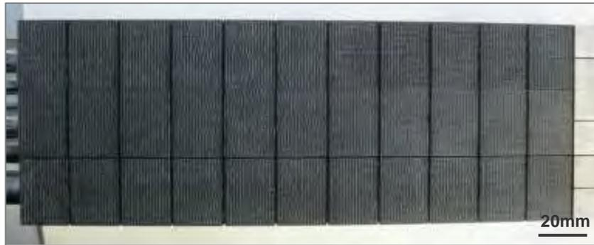
Fig. 23: Top view of the CFC region of the mono flat tile prototype after slot machining (castellation).
