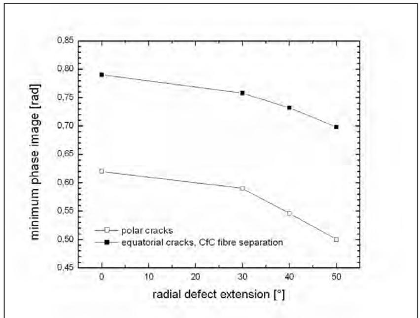
Fig. 11: Dependence of the PPT phase image on the radial defect extensions.
