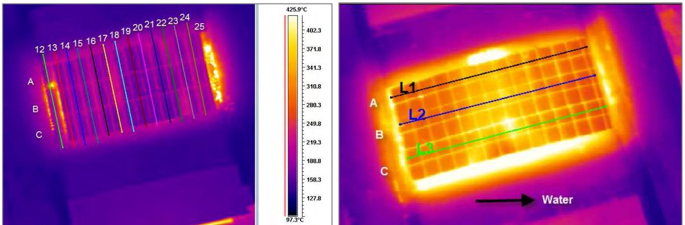
Fig. 18: Surface temperature map of the W region under a heat flux of 5 MW/m<sup>2</sup> (left: monoblock option, right: flat tile option).
