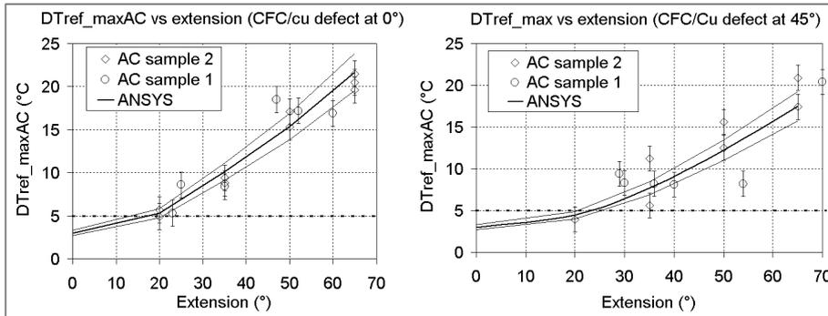
Fig. 14: Comparison between measured and calculated DTref\_Max obtained on top surface for defects at position 0° and 45°.
