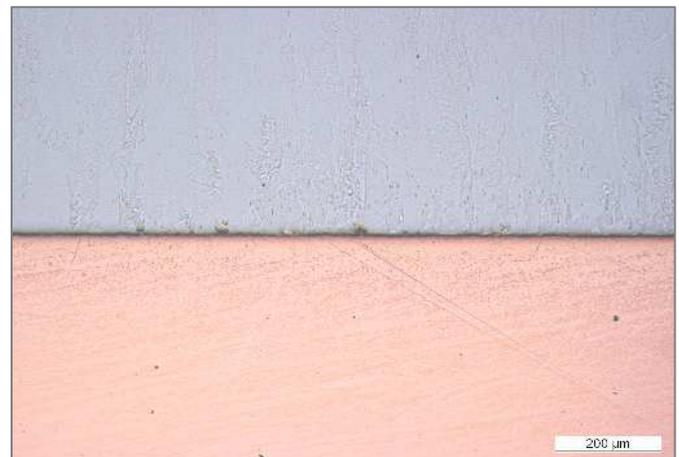
Fig. 8: Cross section of cast W/Cu interface.
