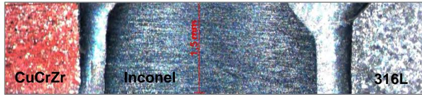
Fig. 6: Cross section of electron beam welded CuCrZr/Inconel/316L transition.
