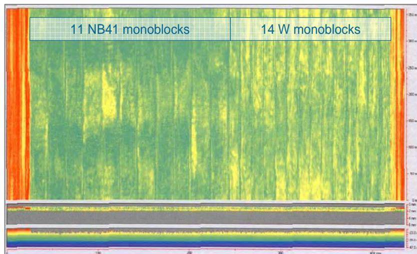
Fig. 9: Ultrasonic scan of the HIP interface of CFC/Cu and W/Cu monoblock armour to cooling tube.
