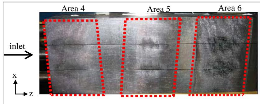
Fig. 19: Zoom on the CFC monoblock surface after testing.
