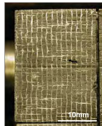
Fig. 25: Crack in the CFC monoblock “A1”, observed after 1000 cycles at 20 MW/m<sup>2</sup>.
