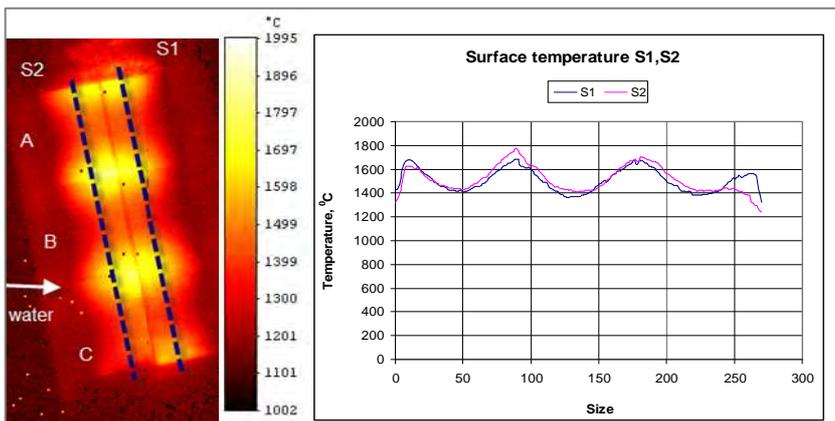
Fig. 24: Surface temperature cartography of CFC monoblocks at 20 MW/m<sup>2</sup> heat flux. S1 and S2 show a maximum T<sub>surf</sub> of ~1800 °C (T<sub>calc</sub> = 1780 °C).
