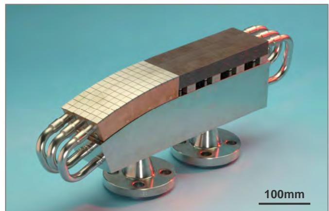
Fig. 5: IVT mono flat tile qualification prototype.
