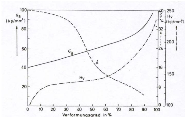
Figure 3: Mechanical properties of Niobium as function of deformation degree [8]
