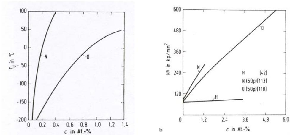
Figure 4: Influence of interstitial elements on the hardness (left) and the brittle/ductile transition temperature (right) of Niobium [11]
