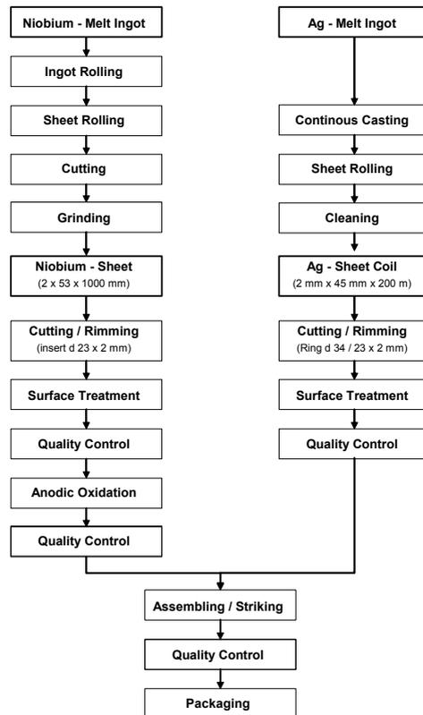
Figure 4: Production steps for manufacturing of bi-metallic Ag/Nb coins from the melt ingot to the coin.
