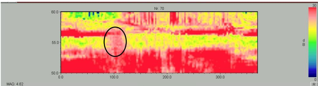
Figure 12: Documentation of the UT inspection of the joining of the tube to the component. The horizontal axis scales the angle of inspection, the vertical axis the depth range.
