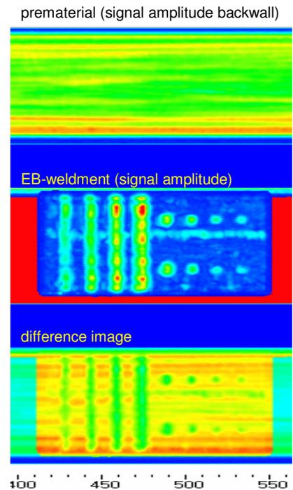
Figure 11: UT result of the test body in Figure 10.
