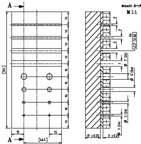
Figure 10: Drawing of a test body containing artificial defects.
