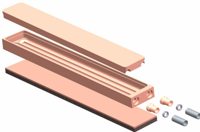
Figure 1: Exploded view of a typical design of a plasma facing component.
