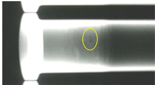
Figure 4: X ray image of an electron beam welded connection tube containing a defect indication.
