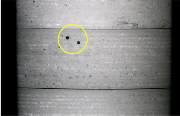
Figure 7: Detection of pores in the copper layer attached to the CFC by RT method.
