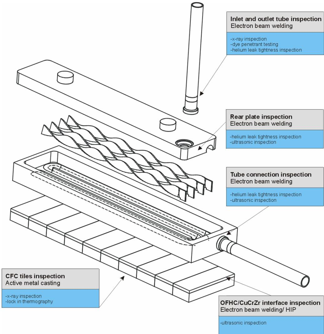
Figure 2: Overview of the material joints of the first wall component focused by the NDT concept.
