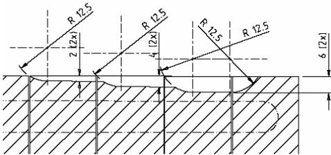
Figure 13: Scetch of the test defects inserted in a finished component.
