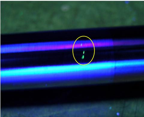
Figure 3: Picture of a PT defect indication detecten on an electron beam welded connection tube.
