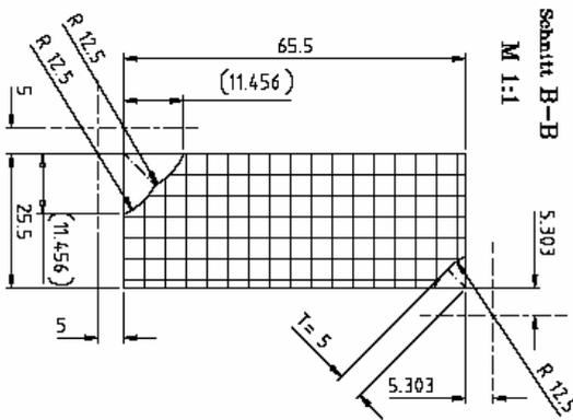
Figure 8: Drawing of a test body containing artificial defects.
