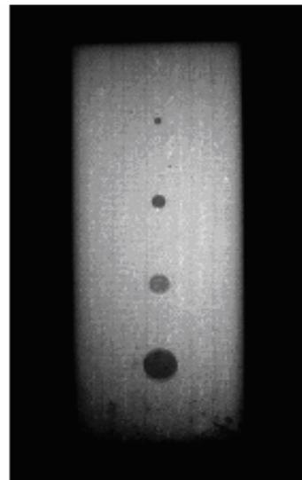
Figure 5: Drawing of a test body containing artificial defects.
