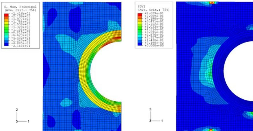
**Fig. 8** Predicted distribution of the maximum principal stress (*left*) and the state dependent variable corresponding to accumulated damage in high heat flux direction in the tensile regime (*right*) after active metal casting, machining, and hot isostatic pressing including de-canning.
