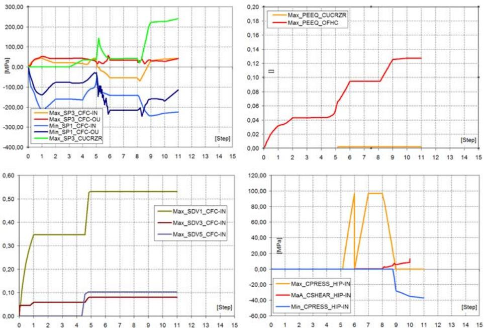
**Fig. 6** Predicted temporal evolution of stress and strain measures, damage relevant parameters, and interfacial stress components for several material points of interest during the active metal casting, machining, and hot isostatic pressing of a divertor component by using finite element modelling.
