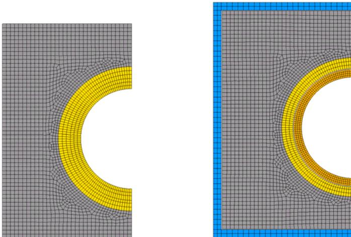
**Fig. 4** Finite element models configured for active metal casting (*left*) and hot isostatic pressing (*right*) of a CFC monoblock: Grey colour indicates the CFC section, yellow colour represents the OF-Cu section, brown colour stands for the CuCrZr tube section, and blue colour represents the section for the steel can, respectively.
