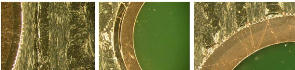
**Fig. 2** Metallographic sections indicating deterioration of CFC sections (*left*), decohesion at the OF-Cu/CuCrZr interface, i.e. the HIP interface (*middle*), and decohesion at the CFC/OF-Cu interface, i.e. the AMC interface (*right*); Cracking in the CuCrZr tube sections is not shown.
