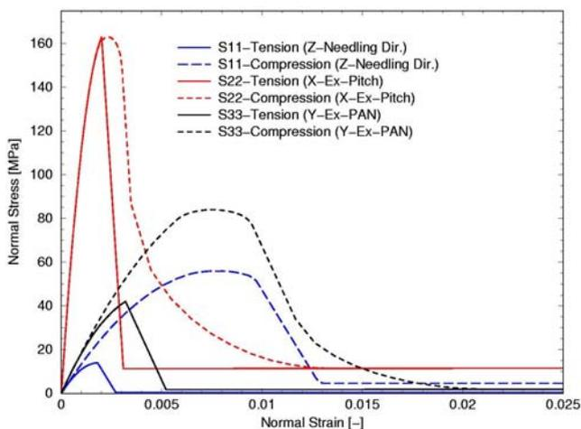
**Fig. 5** Uniaxial stress-strain characteristics of CFC grade NB31 in different directions X (Ex-Pitch), Y (Ex-PAN), and Z (Needling) for the tensile (solid lines) and the compressive (dashed lines) regime, respectively, as used in the FE-models.
