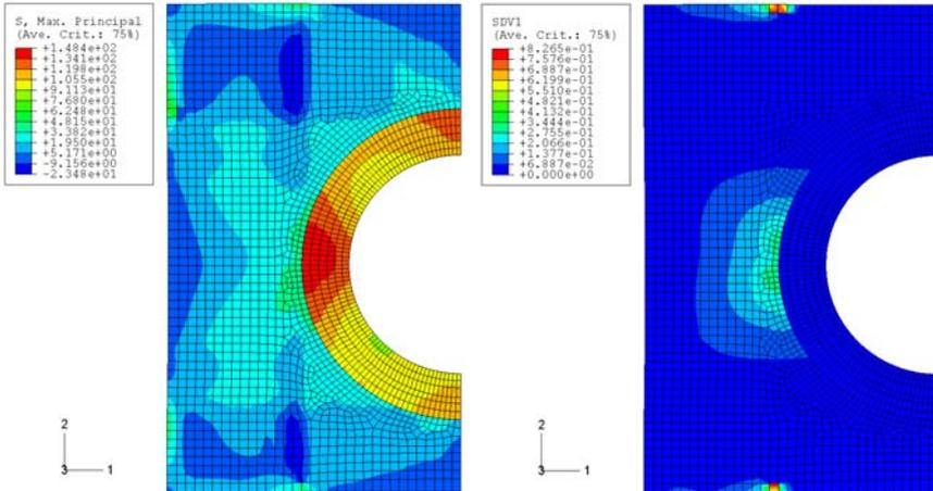
**Fig. 7** Predicted distribution of the maximum principal stress (*left*) and state dependent variable corresponding to accumulated damage in high heat flux direction in the tensile regime (*right*) after active metal casting prior to machining.
