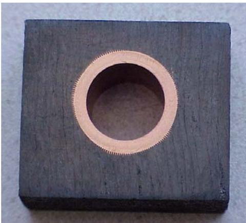
**Fig. 10** Cross section of a CFC monoblock divertor component showing the CFC section, the OF-Cu section, and the CuCrZr-tube section, respectively; the component is processed successfully via active metal casting, machining, and hot isotstatic pressing.
