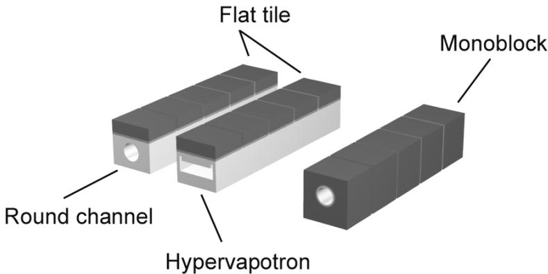
**Fig. 1** Sketches of flat tile (*left*) and monoblock (*right*) components, respectively, as used in nuclear fusion divertors.
