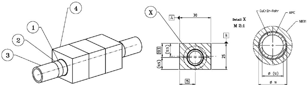
**Fig. 3** Sketch of a CFC monoblock divertor component with section 1 representing the CuCrZr tube, section 2 showing the Ni region, section 3 representing the 316L steel adapter, and section 4 showing the CFC block of grade NB31 (*left*), and corresponding cross section (*middle to right*). Note that the steel can for the HIP procedure is not shown.
