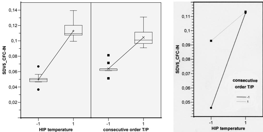
**Fig. 9** Predicted response graph for the state dependent solution variable SDV5 representing accumulated damage in the CFC section in out of plane direction (*left*) and predicted interaction graph for the influence parameters HIP temperature and consecutive order of HIP temperature and pressure loading, respectively, with respect to SDV5 (*right*) by using the FEA-DoE approach.
