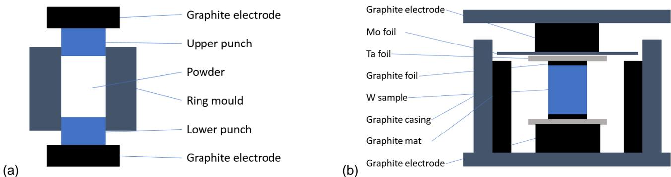
Figure 2: (a) Original setup for direct current sintering. (b) Adapted experimental setup for high temperature emissivity measurements.
