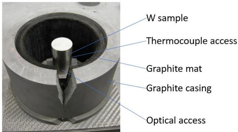
Figure 3: W sample inside the graphite casing and mat.
