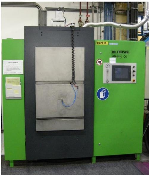
Figure 1: FAST/SPS sintering press DSP 515 from Dr. Fritsch used for the measurements.
