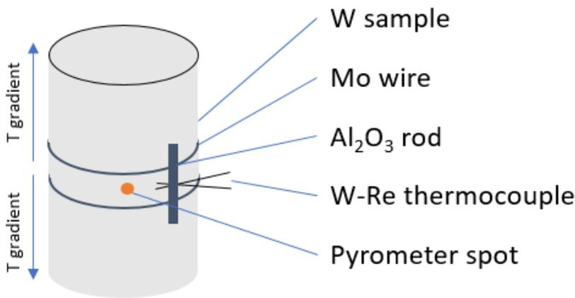
Figure 4: Temperature measurement by thermocouple.
