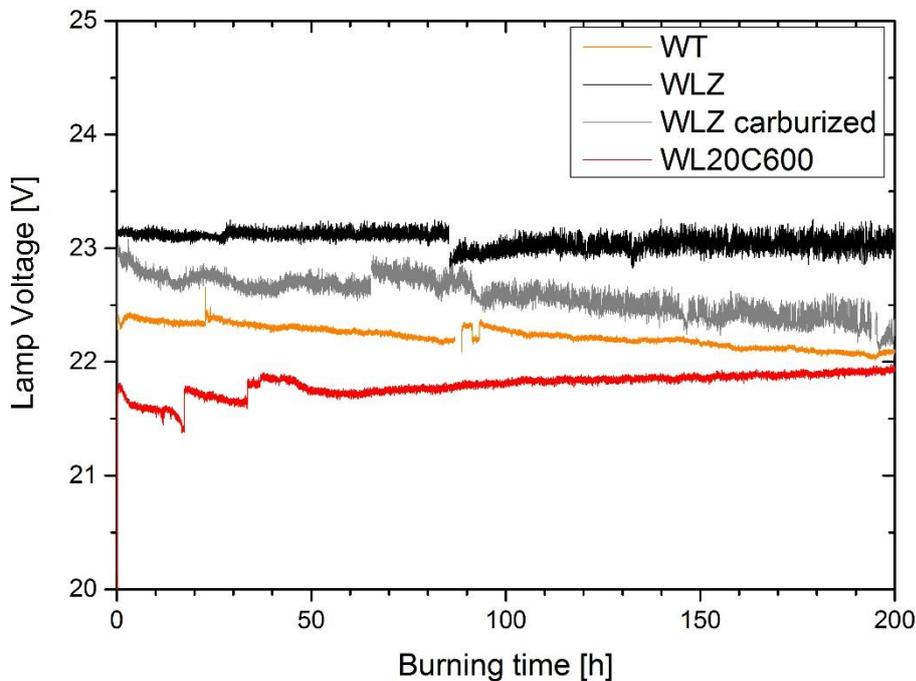
Figure 10: Voltage fluctuation during the first 200 hours of the lamp test as a measure for flickering of 3,5 kW standard lamps containing different cathode materials.
