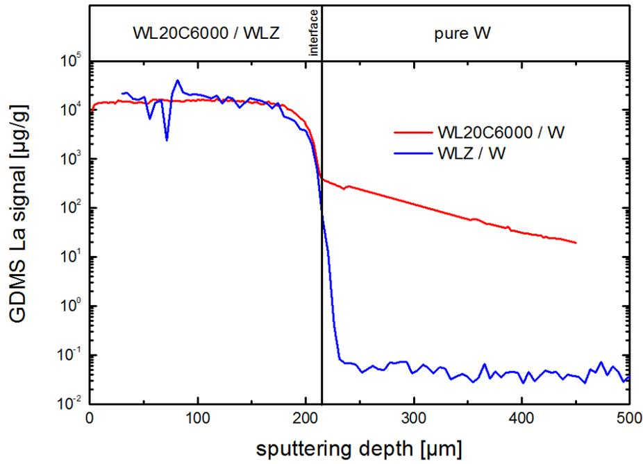
Figure 7: Lanthanum signal of the GDMS measurement through the interface of diffusion couples.
