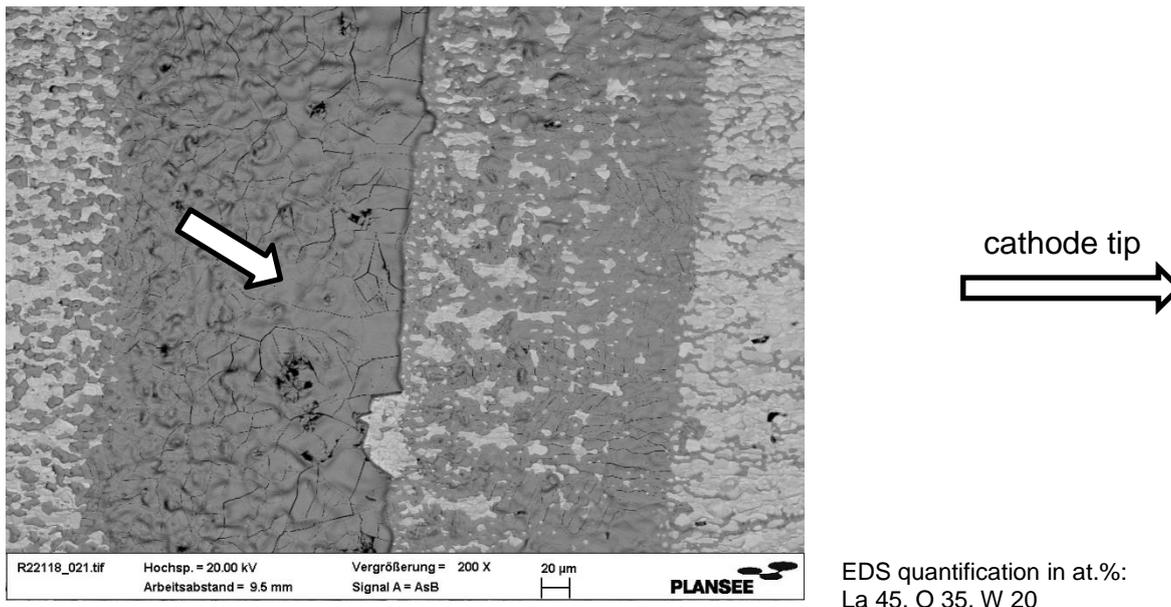
Figure 6: SEM mass contrast image of the emitter deposit after the lamp test of the WLZ cathode shown in Fig. 4–5. The location of EDS is marked by the white arrow.
