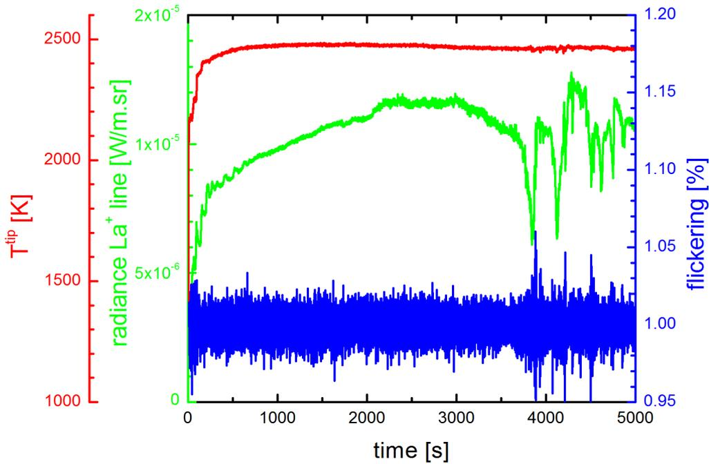
Figure 4: Time-resolved “Bochum Model Lamp” test data obtained from WLZ cathode material.  $T^{\text{tip}}$  (red), the intensity of the  $\text{La}^+$  line close to the tip (green) and the normalized photocurrent (blue) are shown for the first 5000 s of the lamp test.
