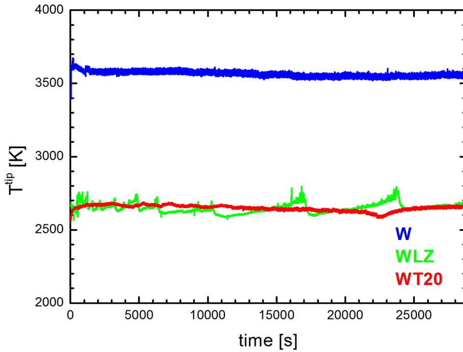
Figure 3: Time-resolved “Bochum Model Lamp” test data obtained from different cathode materials.  $T^{\text{tip}}$  is shown for the whole test duration of 8 h.
