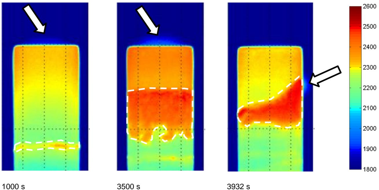
Figure 5: Temperature image of a WLZ cathode at different times. The lamp test data of this cathode is shown in Fig. 4. Temperature determination (K) is based on the emissivity of pure tungsten. A scale for the images is provided by the diameter of cathode which is 1.5 mm. The white arrows indicate the location of the arc spot. The white dashed lines mark the emitter depositis beyond the tip of the cathode.
