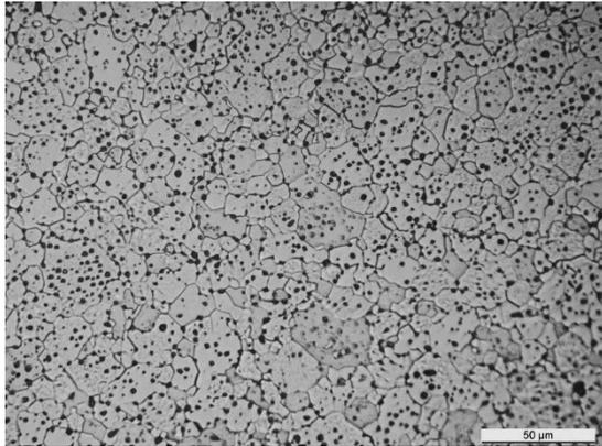
Figure 1: LOM of a metallographic section of WL20C600 in etched condition. The  $\text{La}_2\text{O}_3$  particles can be recognized as black dots.
