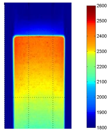
Figure 9: Temperature image of a WL20C600 cathode at 2500 s, for lamp test data see Fig. 8.
