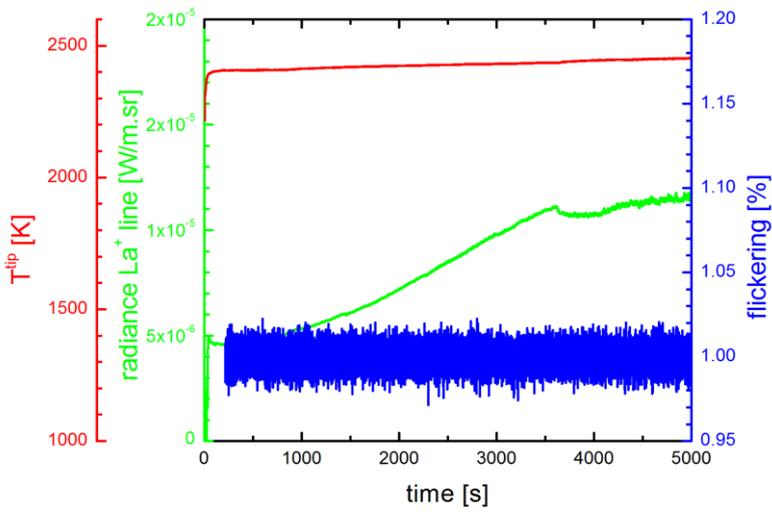
Figure 8: Time-resolved test data obtained from WL20C600 cathode material in the “Bochum Model Lamp”.
