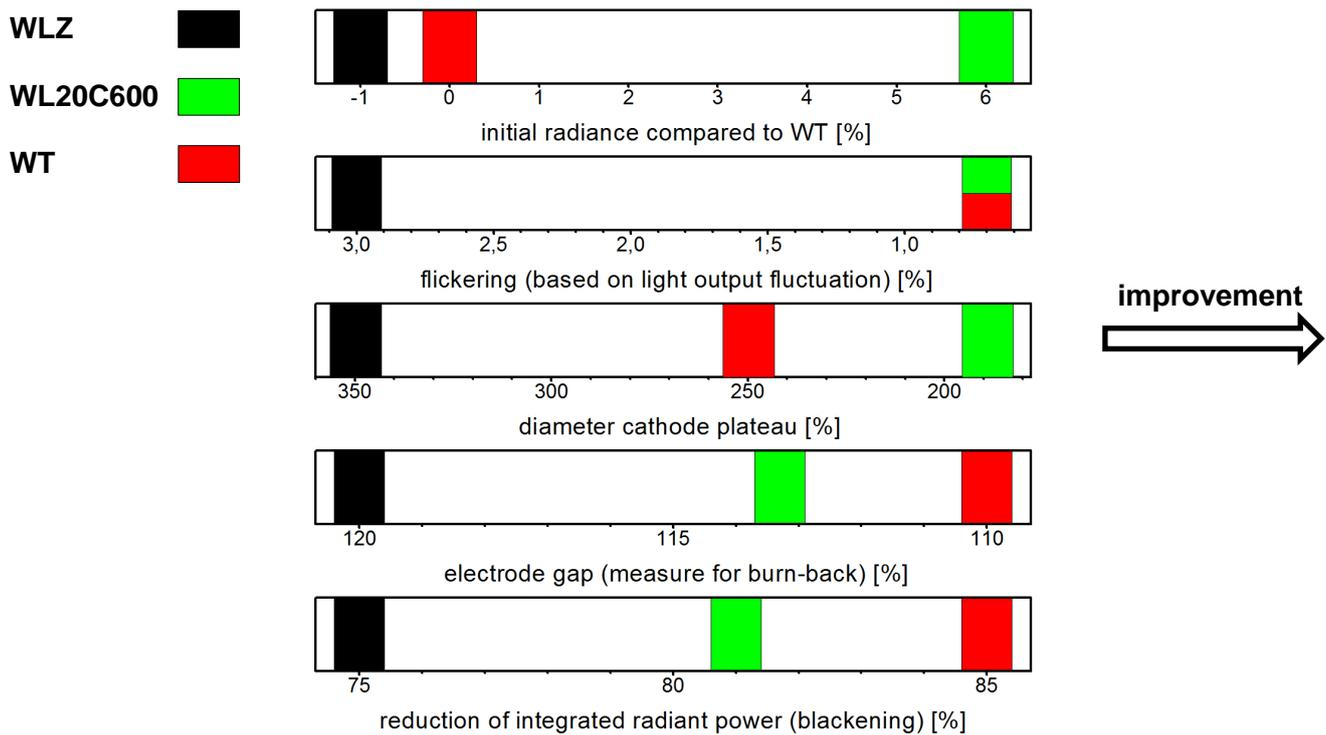
Figure 11: Rating of the cathode materials WLZ (black), WL20C600 (green) and WT (red) for all target quantities regarded for industrial application of a 3,5 kW standard mercury discharge lamp. The scale definition of the individual axes of abscissae enables the visualization of improvement as a shift towards the right side for all target quantities.
