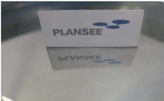
Figure 5: Mirror-like surface of a surface conditioned pressed-sintered Mo sample.
