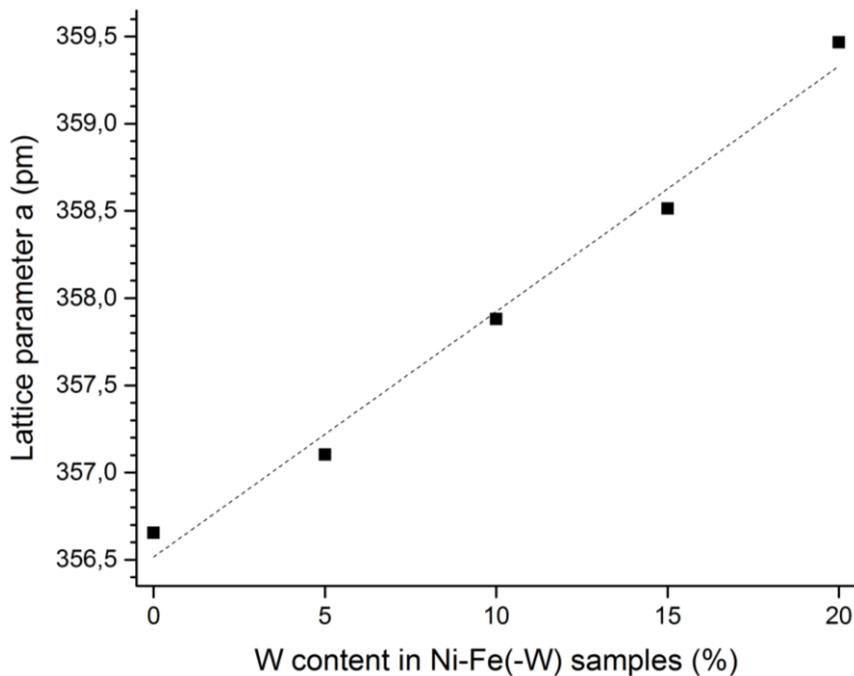
Figure 5: Lattice parameters of Ni-Fe(-W) samples with varying tungsten contents
