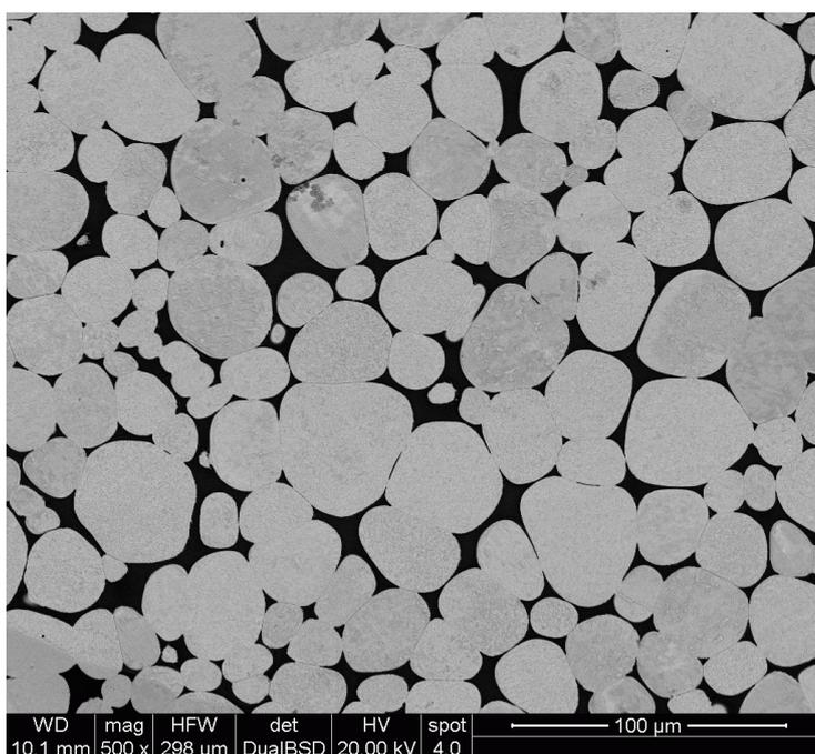
Figure 1: Typical structure of a 95W-Ni-Fe heavy alloy (BSE image, tungsten particles are bright, binder phase is dark)
