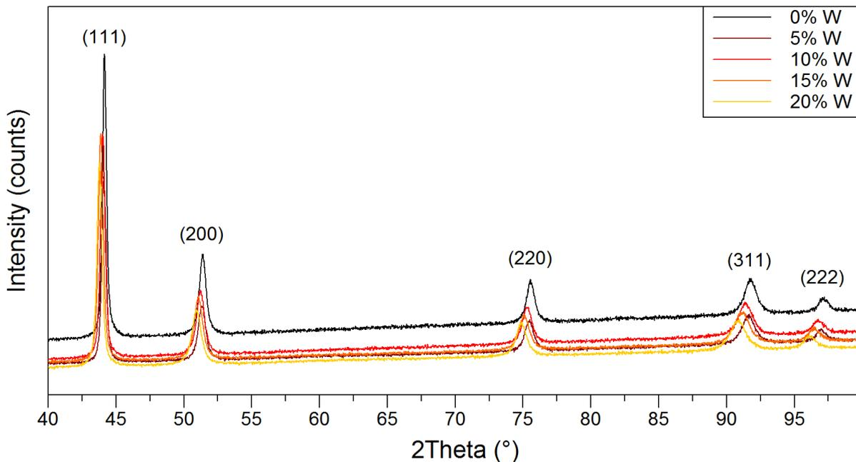
Figure 4: X-ray diffractograms of Ni-Fe(-W) samples with varying tungsten contents
