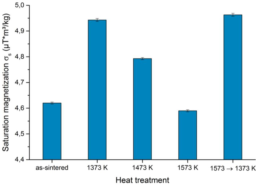
Figure 2: Weight-specific saturation magnetization of *Densimet 180*<sup>®</sup> samples after different vacuum heat treatments
