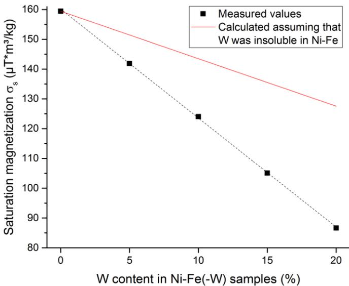
Figure 3: Weight-specific saturation magnetization of Ni-Fe(-W) samples with varying tungsten contents
