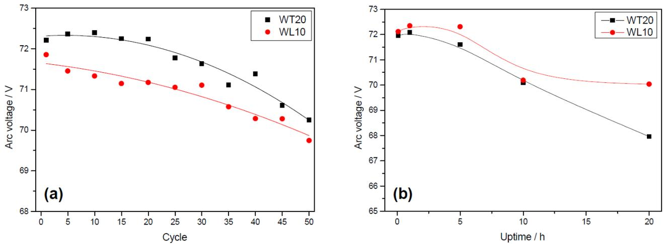
Figure 1: Arc voltage as a function of (a) number of cycles and (b) uptime for the electrode materials WT20 and WL10.
