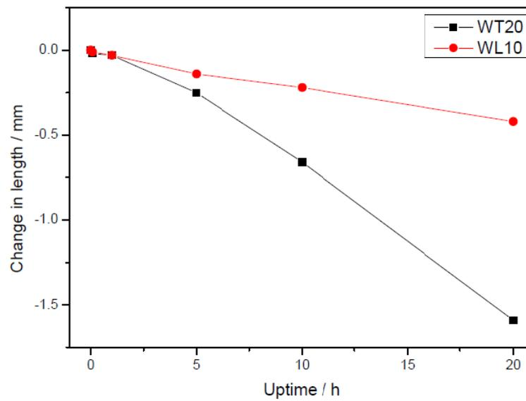
Figure 4: Change in cathode tip length as a function of uptime for the electrode materials WT20 and WL10 .
