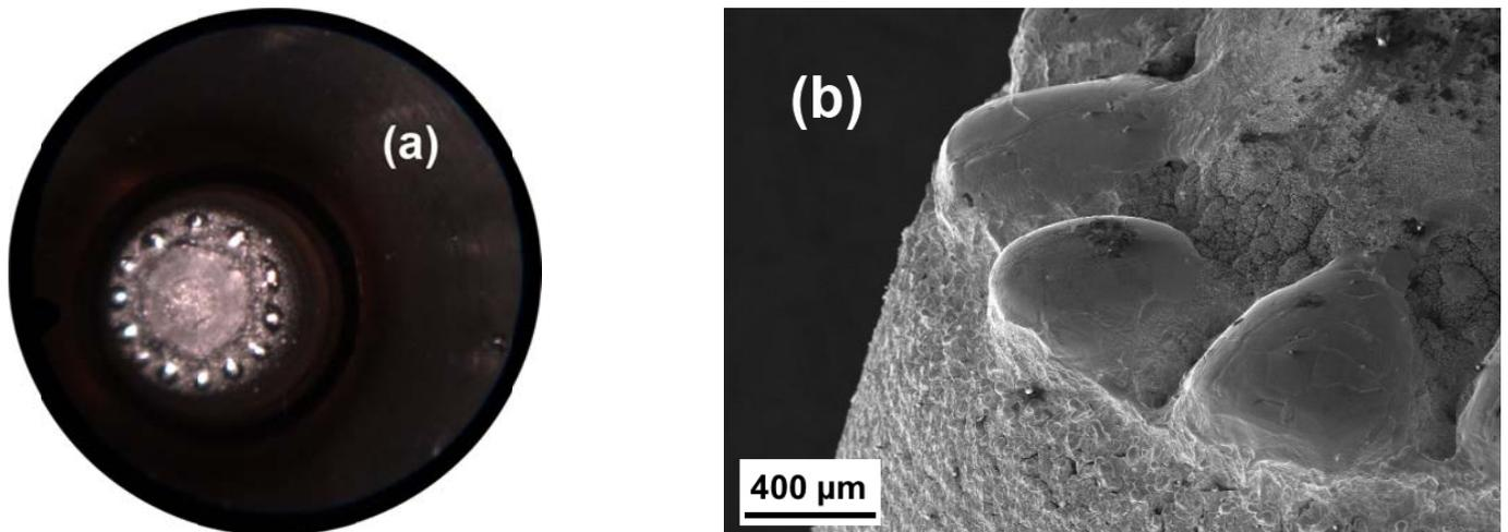
Figure 5: WT20 cathode after (a) 20 ignitions (endoscope) and (b) after 50 ignitions (SEM).
