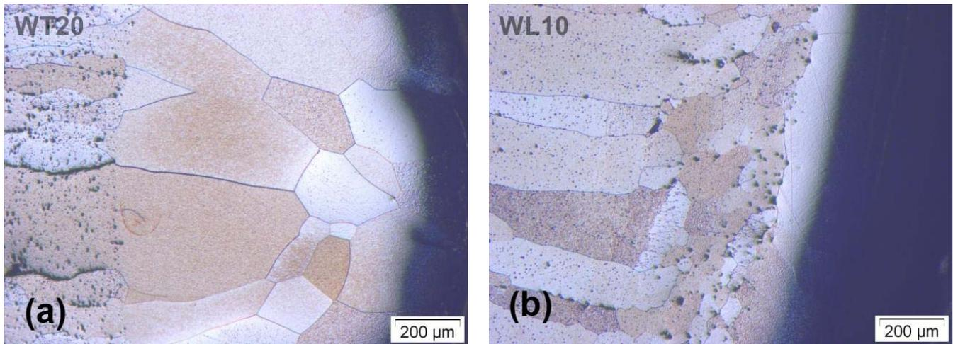
Figure 7: Optical micrographs of the structure at the cathode tip region. (a) WT20, (b) WL10.
