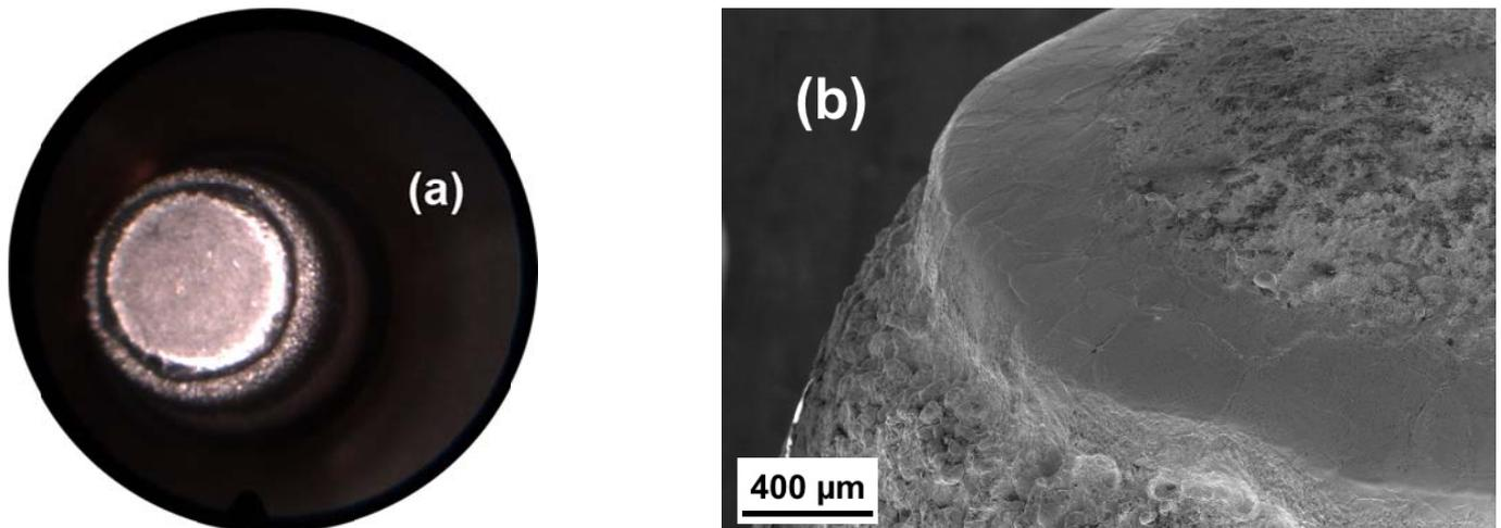
Figure 6: WL10 cathode after (a) 20 ignitions (endoscope) and (b) after 40 ignitions (SEM).
