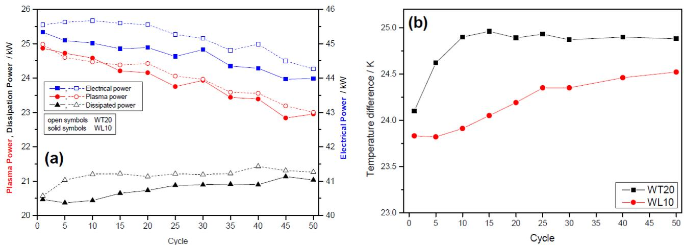
Figure 2: (a) Electrical, plasma and dissipated power and (b) temperature difference of cooling water at inlet and outlet as a function of number of cycles for the electrode materials WT20 and WL10.
