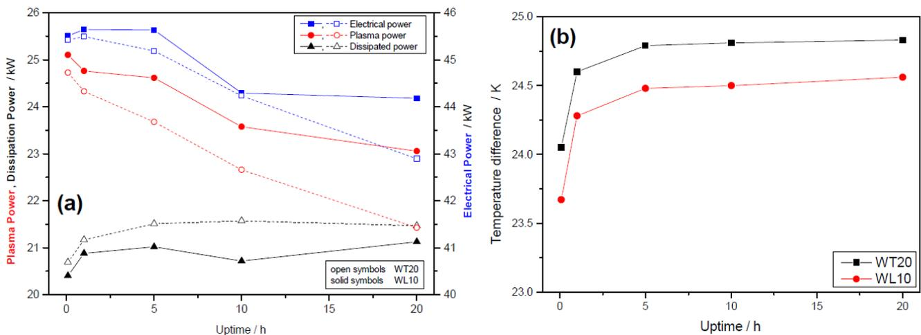
Figure 3: (a) Electrical, plasma and dissipated power and (b) temperature difference of cooling water at inlet and outlet as a function of uptime for the electrode materials WT20 and WL10.
