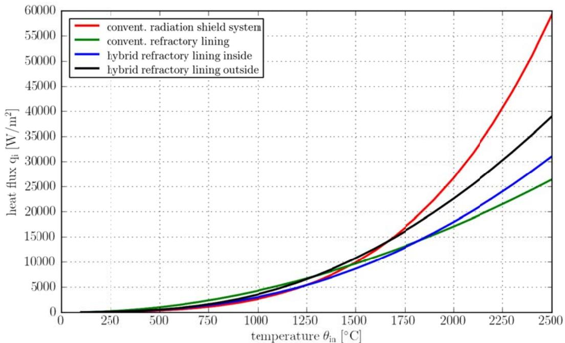
Figure 3: Predicted heat flux of the four thermal insulation systems.
