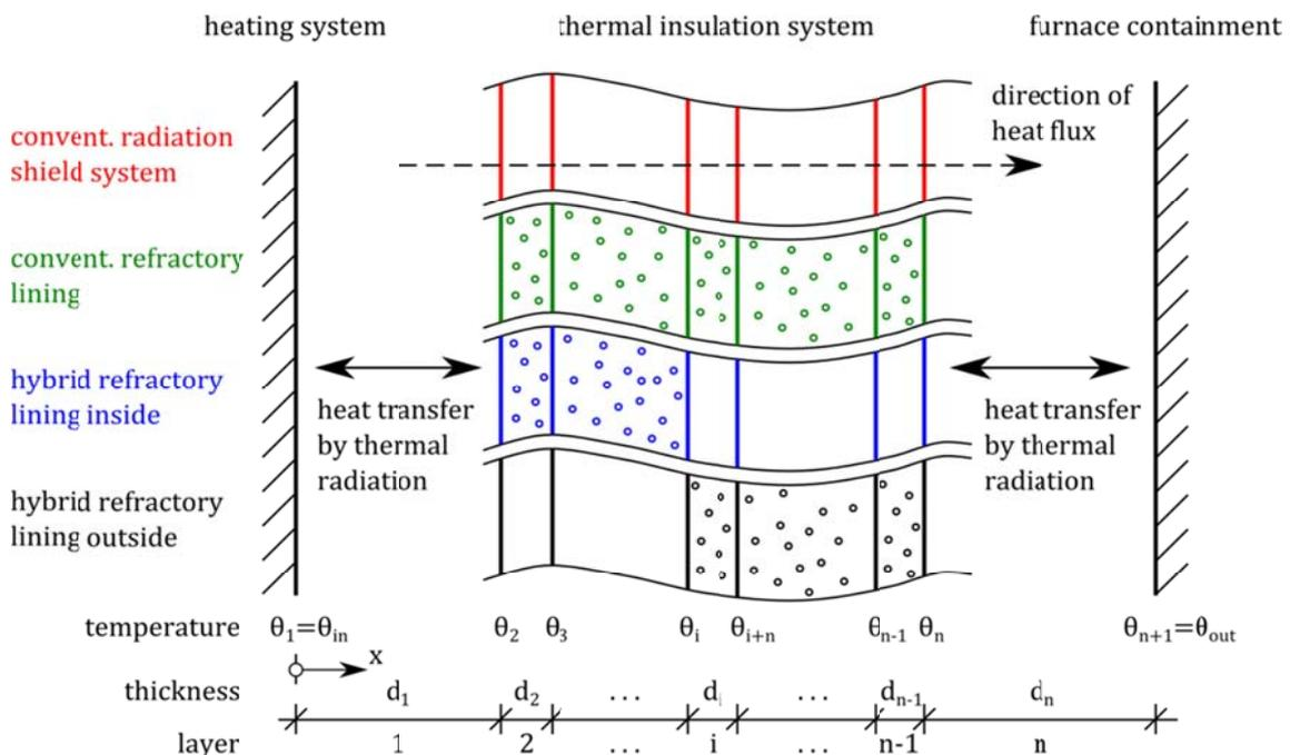
Figure 2: Schematical design of the numerical models.
