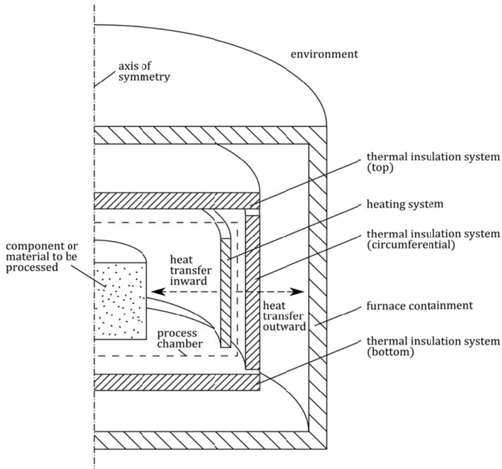
Figure 1: Schematical design of a high-temperature furnace of cylindrical shape.
