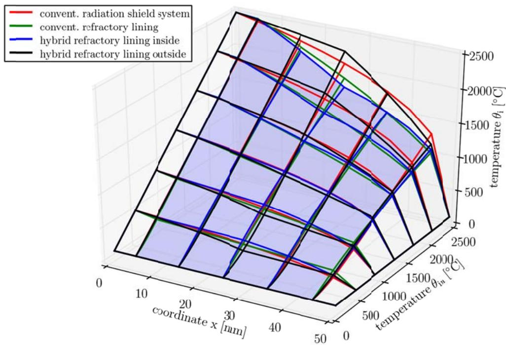
Figure 4: Predicted temperature distribution in the thermal insulation of the four thermal insulation systems for  $\theta_{in} = [100, 500, 900, 1300, 1700, 2100, 2500]$  [°C].
