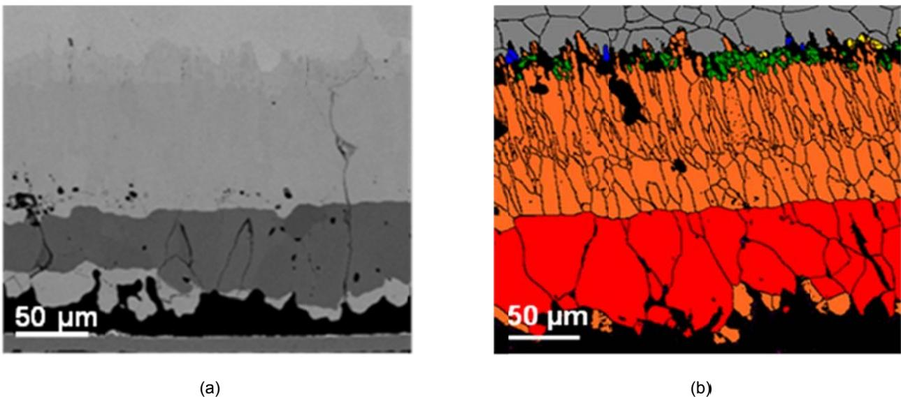
Figure 6:(a) SEM-BSE images of a cross section through a SIBOR<sup>®</sup>-coated Mo sample after 10 h at  $1650^\circ\text{C}$  in air. (b) EDS-EBSD phase assignment with grain boundaries (local orientation difference  $>5^\circ$ ). Color code: red- $\text{MoSi}_2$ ; orange- $\text{Mo}_5\text{Si}_3$ ; yellow- $\text{Mo}_3\text{Si}$ , blue- $\text{Mo}_2\text{B}$ ; green- $\text{Mo}_5\text{SiB}_2$ ; violet- $\text{SiO}_2$ ; grey-Mo; black: grain boundaries.
