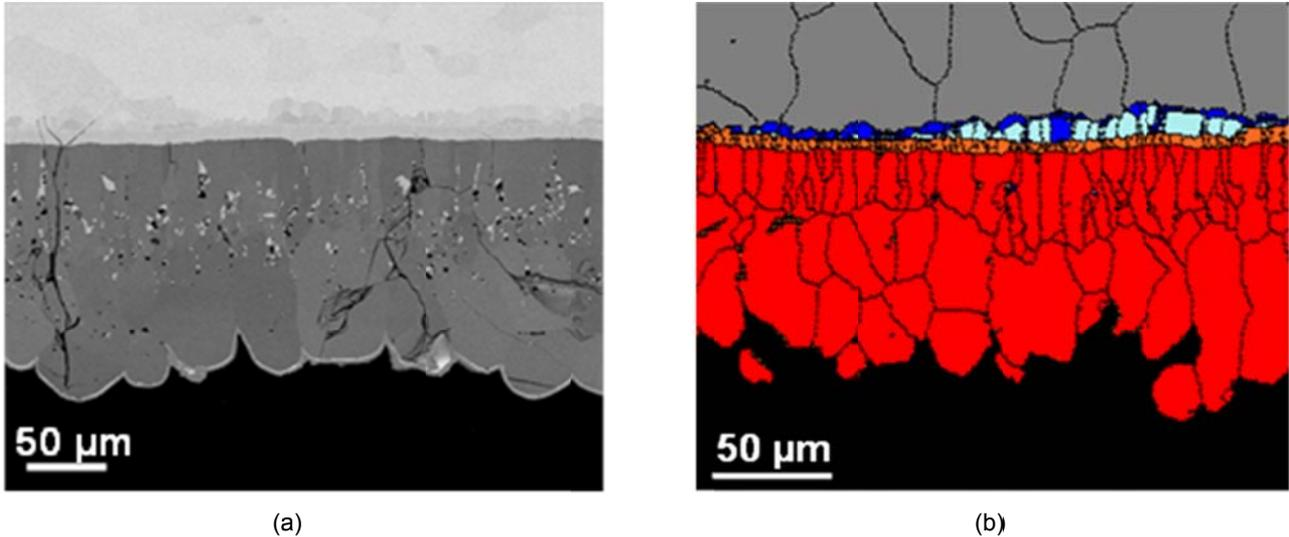
Figure 1: (a) SEM-BSE image of a cross-section through a SIBOR<sup>®</sup>-coated Mo sample after hydrogen annealing. (b) EDS-EBSD phase assignment of (a) including grain boundaries (local differences in orientation  $>5^\circ$ ). Color code: red- $\text{MoSi}_2$ ; orange- $\text{Mo}_5\text{Si}_3$ ; light-blue- $\text{MoB}$ ; blue- $\text{Mo}_2\text{B}$ ; grey-Mo; black: grain boundaries.
