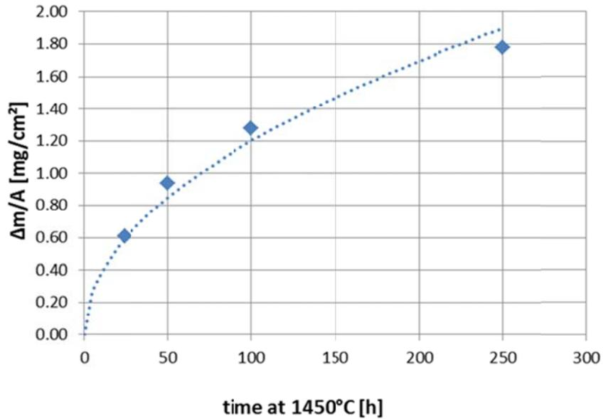
Figure 5: Mass gain of SIBOR<sup>®</sup> samples at  $1450^\circ\text{C}$  in air.
