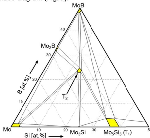
Figure 7: Isothermal section through the Mo-rich corner of the Mo-Si-B phase diagram at 1450°C.
