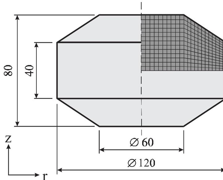
Figure 6. Sketch of the tapered disk sample with finite element mesh.
