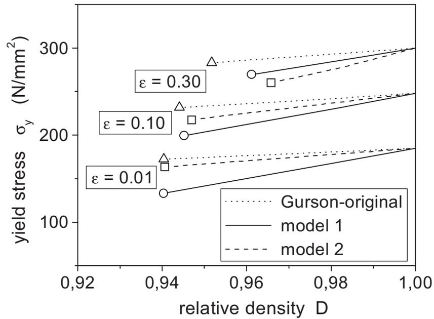
Figure 4. Yield stress of the porous metal versus relative density for different levels of plastic strain; original Gurson model (with  $q_1 = q_2 = 1$ ) compared with the modified Gurson model (model 1) and the Gologanu model (model 2).
