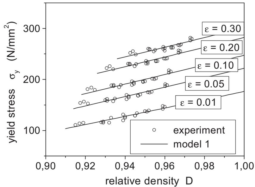
Figure 1. Yield stress of the porous metal versus relative density for different levels of plastic strain; experiments (uniaxial compression) compared with the modified Gurson model (model 1).
