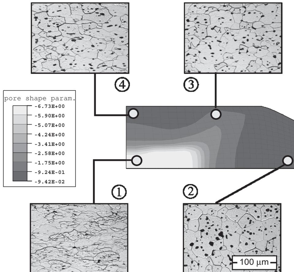
Figure 8. Pore shape parameter S for the first stroke calculated with the Gologanu model (model 2), together with four optical micrographs.
