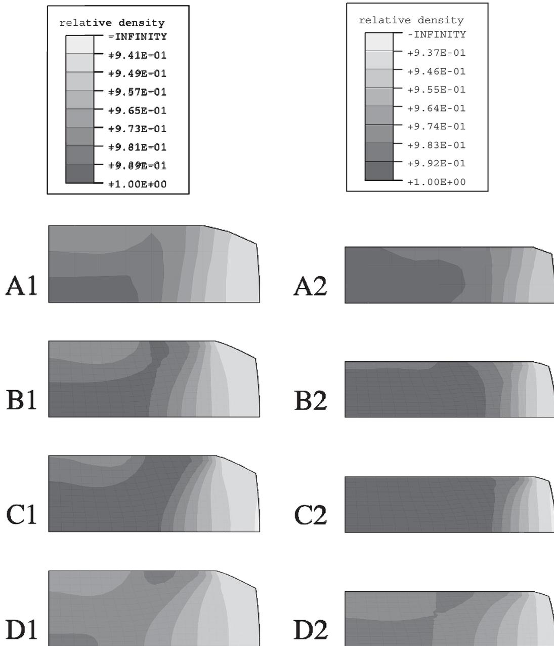
Figure 7. Density distribution for the first stroke (left side: A1 - D1) and for the second stroke (right side: A2 - D2). Comparison of the measured values (A1 and A2), the modified Gurson model (model 1: B1 and B2), the Gologanu model (model 2: C1 and C2) and the original Gurson model (with  $q_1 = 1.5$  and  $q_2 = 1$ ) (D1 and D2).
