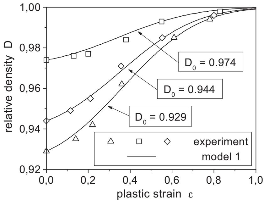
Figure 2. Density evolution in uniaxial compression for different initial densities; experiments compared with the modified Gurson model (model 1).
