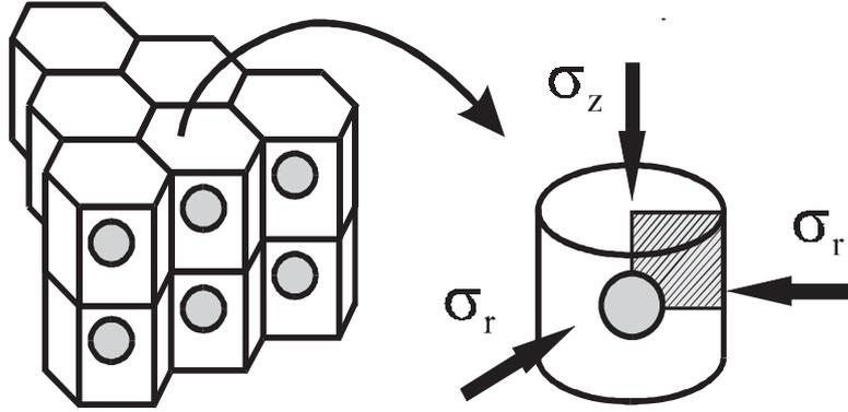
Figure 3. Sketch of regular pore arrangement and the extraction of a axisymmetric unit cell.
