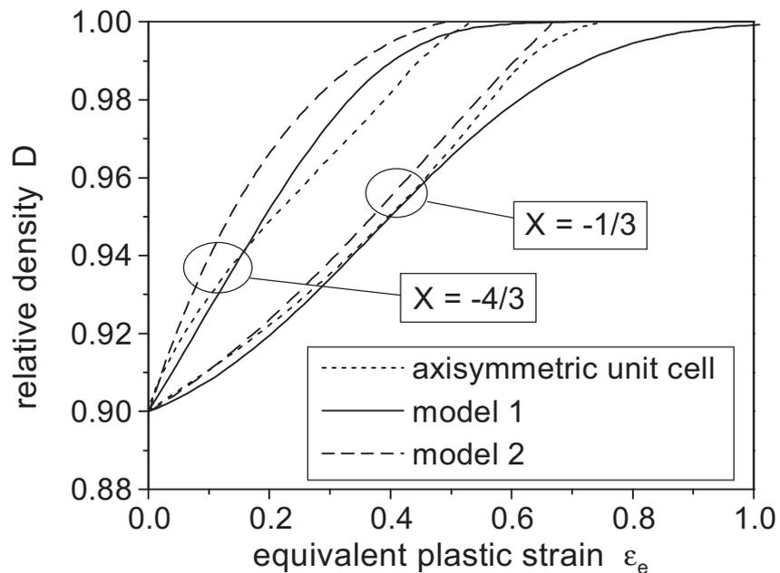
Figure 5. Density evolution for different triaxialities; comparison between axisymmetric unit cell calculations, the modified Gurson model (model 1) and the Gologanu model (model 2).
