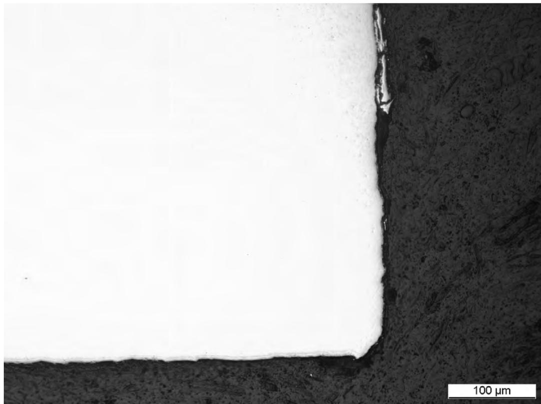
Fig. 3: Optical light micrograph of a cross section of W after 168 h in molten Zn at 500°C (HCl etched )
