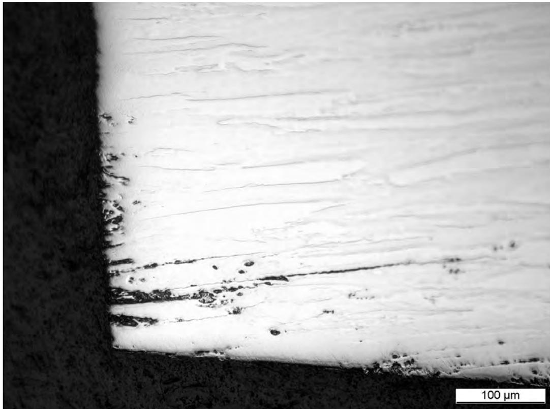
Fig. 2: Optical light micrograph of a cross section of Mo after 168 h in molten Zn at 500°C (HCl etched)
