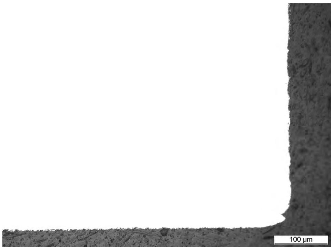
Fig. 4: Optical light micrograph of a cross section of MoW after 168 h in molten Zn at 500°C (HCl etched)
