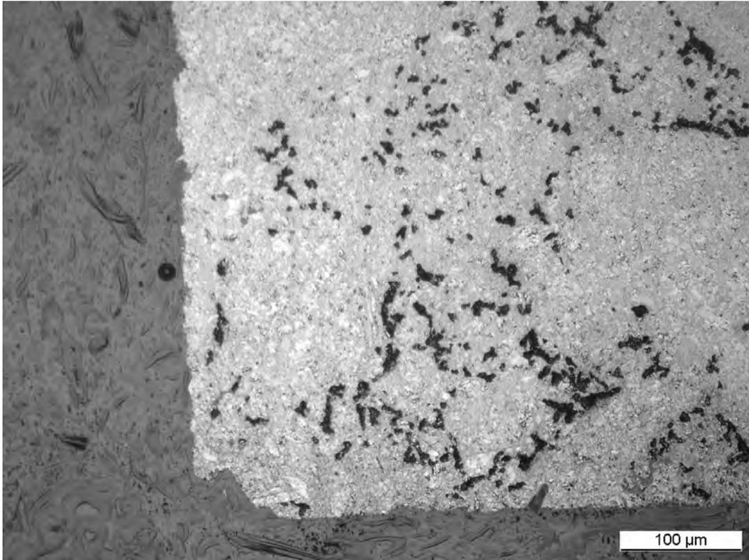
Fig. 5: Optical light micrograph of a cross section of graphite after 168 h in molten Zn at 650°C (HCl etched)
